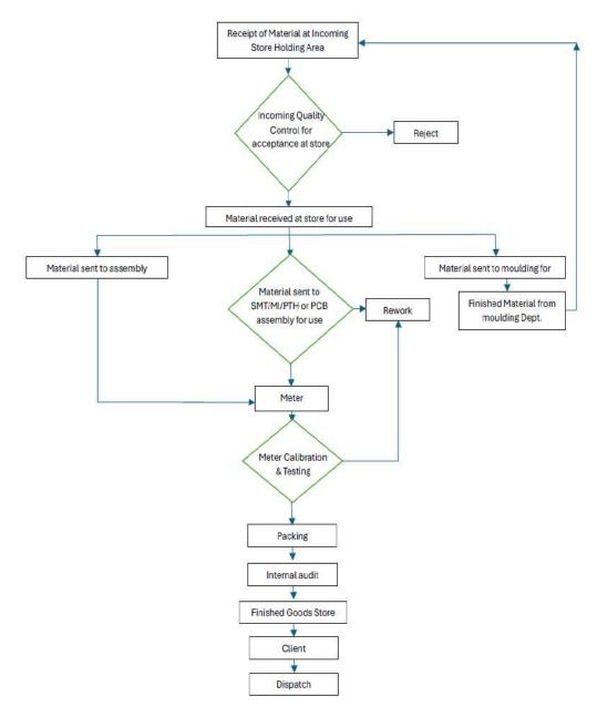
The flowchart above outlines the production and quality assurance process for energy meters, from the receipt of materials to the final dispatch to clients. Step-by-step explanation of the same is provided below:
